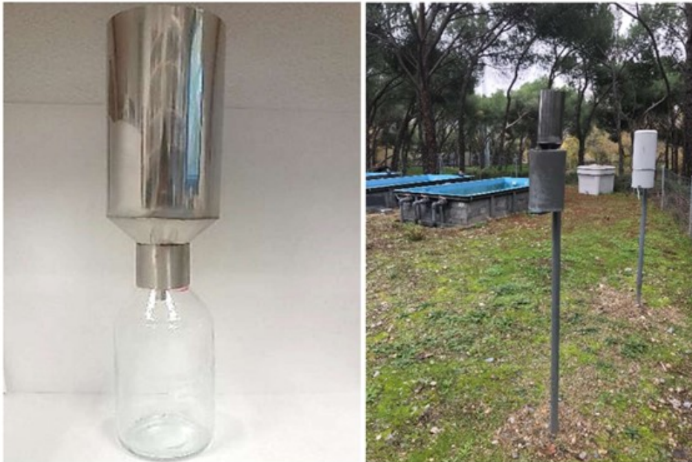
Figure S1: Bespoke collector used and field set-up. (Photo taken in sampling point 3.)
